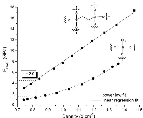
**Figure 1.** Young's modulus for MSSQ-SiO<sub>2</sub> and Et-OCS films as a function of density.
